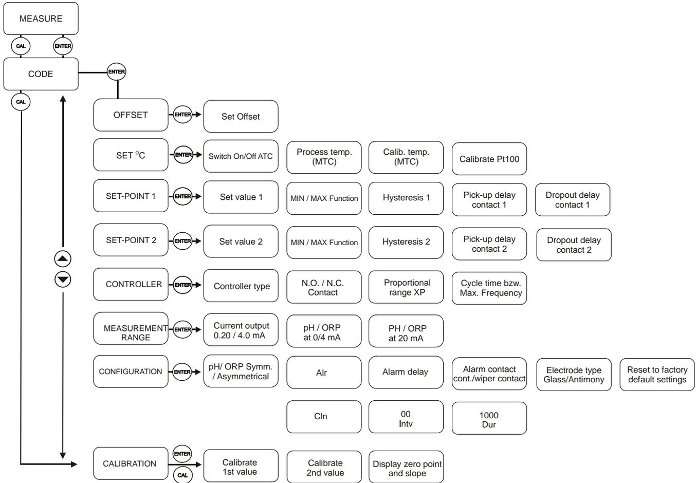
The controller offers two levels of password protection: (1) for direct access to calibration function and (2) for setting or editing specific controller parameters or functions in the SETUP mode to suit individual requirements.
