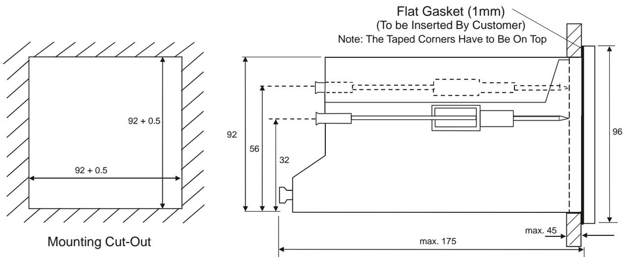
The field-tested control panel housing is 96 x 96 mm; with protection class IP 54 (front).
