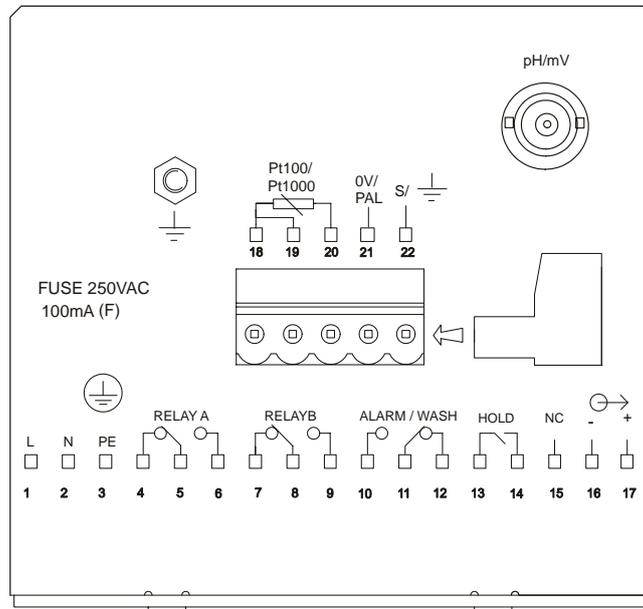
**Important:** The Alarm relay functions as an “Active Low” device i.e. it switches OFF under Alarm condition. Therefore, the Alarm display device should be connected to the ‘NC’ contacts of the relay (11 and 12). In the Wash mode, the relay works on a positive mode. Therefore, the Wash device should be connected to contacts 10 and 11.
