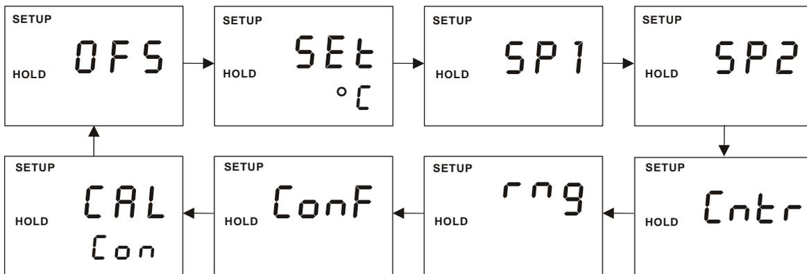
The set-up parameters can be viewed or changed by entering a security code. See section 5.2 for security code information.
