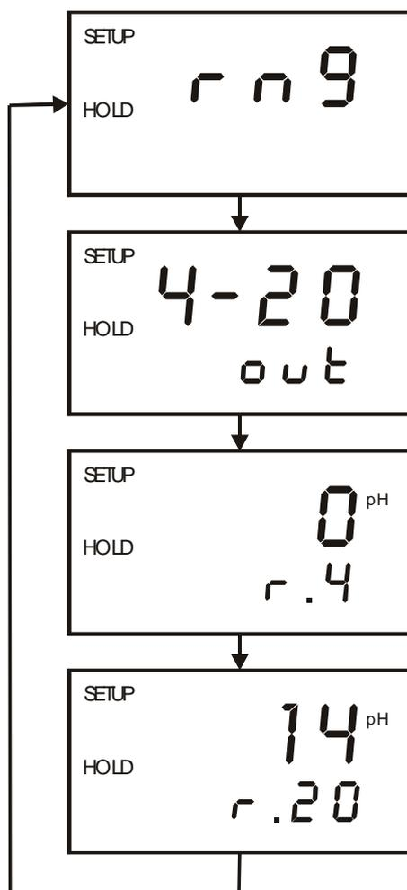
This sub-function lets you set the controller current output range of this unit.
