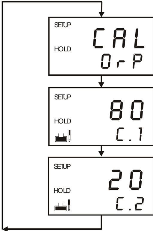
To calibrate the controller for ORP %:
