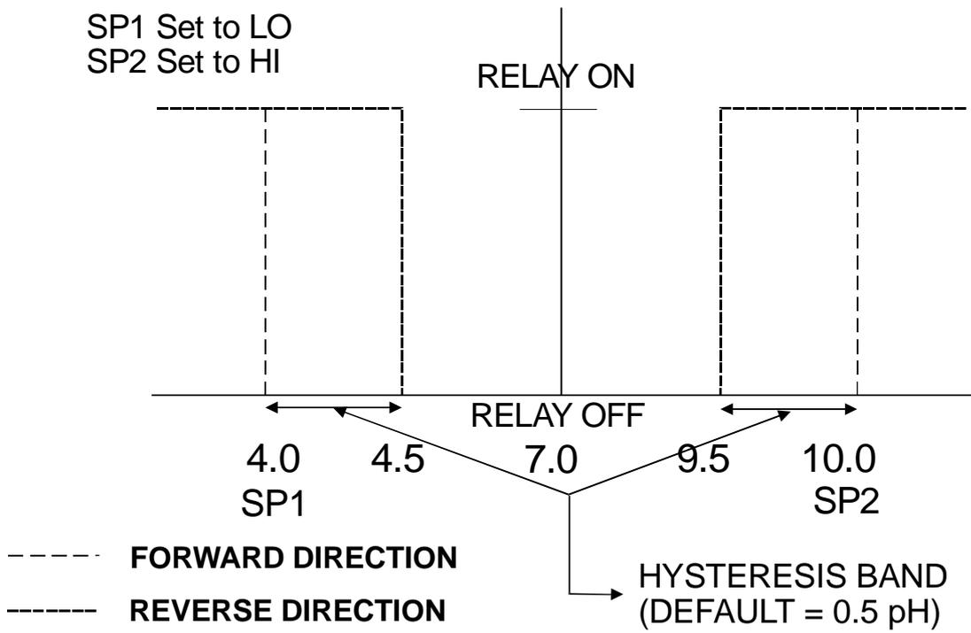
The controller relay activates when the set-point is reached. In the reverse direction, it does not de-activate when the value reaches the set-point. Instead, it continues to be active till the value reaches the amount set by the Hysteresis band.
