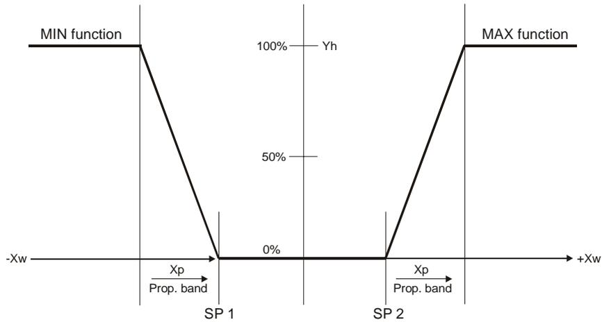
Control characteristic of P-Controller as proportional controller
