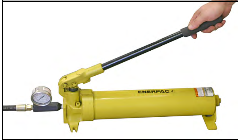
Figure 6-9: Pressurizing the Hydraulic Pump
