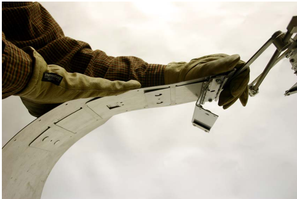
Figure 3-18 Bend the base and/or extension to fully engage the buttons
