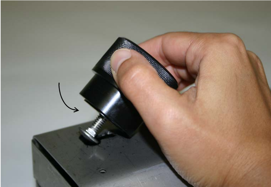
Figure 3-6 Attaching the reflector plate assembly to mounting hardware
