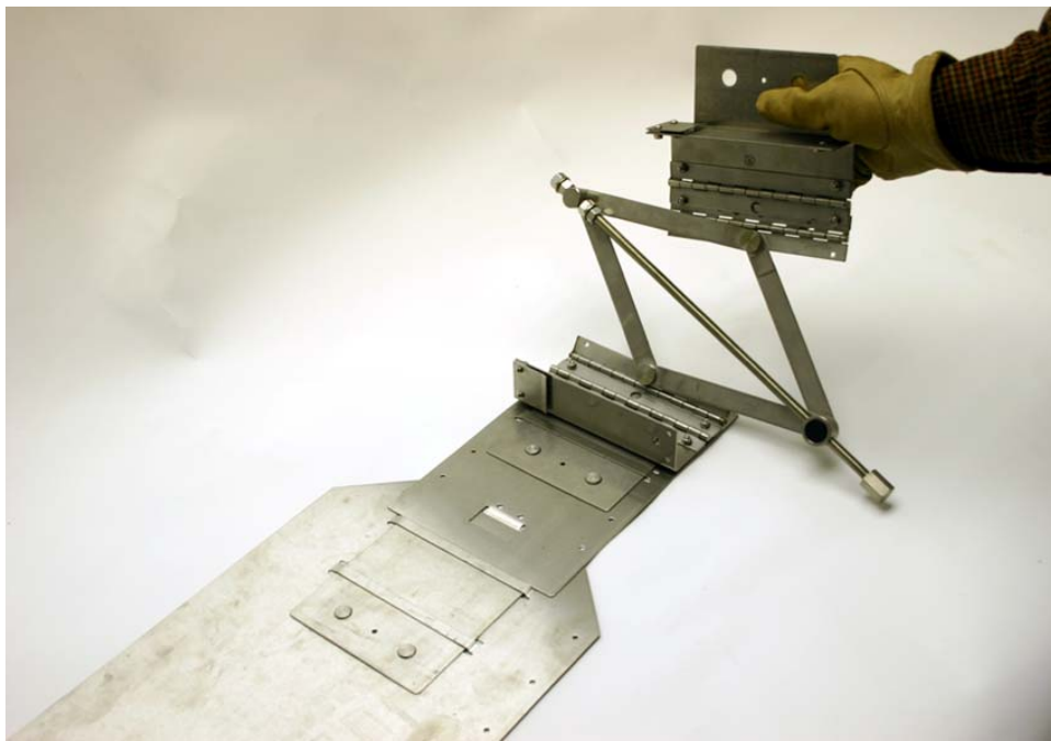
Figure 3-20 Scissors mechanism connected with extension and base
