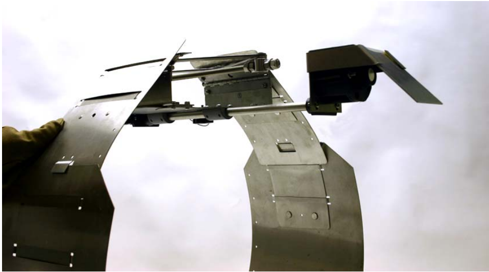
Figure 3-25 Scissor ring and sensor assembled
