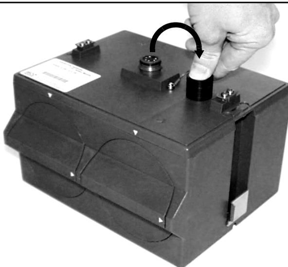
Figure 1-20 Battery Module - Uncapping the Connector
