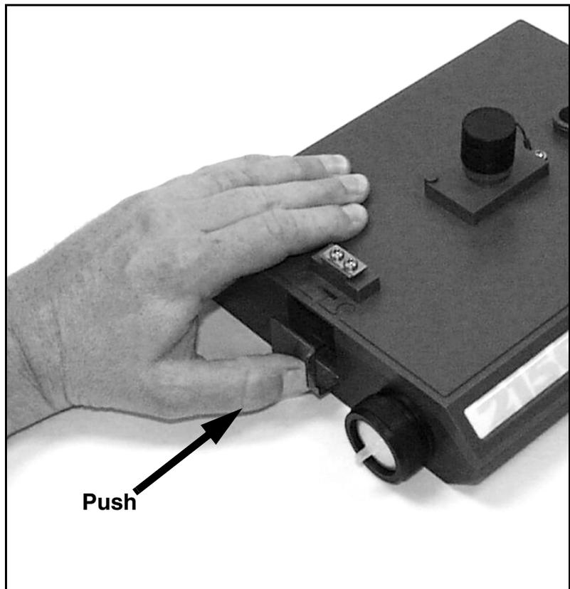
Figure 1-4 Locking the Latch
