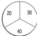
A humidity indicator is mounted inside each battery cap on the Battery Module. The humidity indicators have regions that display 20, 30, and 40 percent humidity levels. Ideally each region should be completely blue. As the desiccant becomes saturated, the humidity levels will increase and the regions turn pink. When the 40 percent region turns pink, the Battery Module is no longer adequately protected and the desiccant must be replaced. Refer to section 6.4 for replacement instructions.
