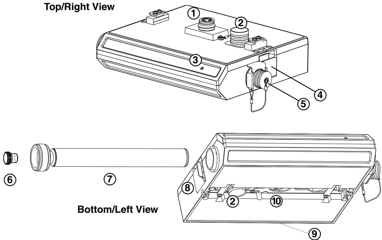
Figure 2-2 Controls, connectors, and indicators – 2150 Flow Module
