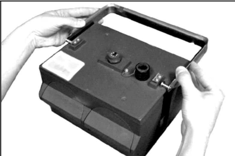
Figure 1-21 Battery Module - Inserting the Handle
