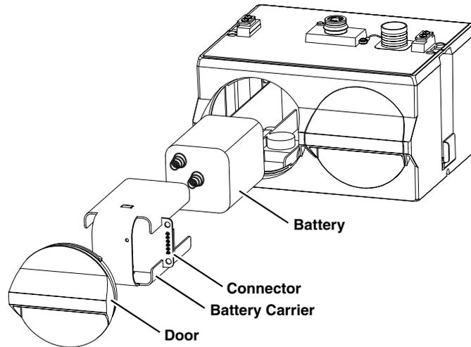
Figure 3-1 Installing a Battery
