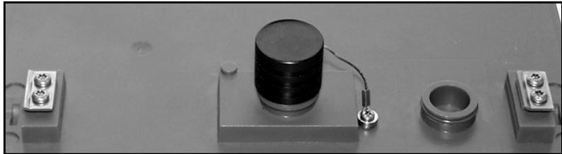
*Figure 1-5 Flow Module - Upper Connector, Capped*
