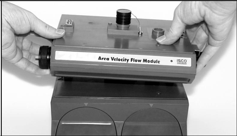
Figure 1-22 Aligning the Modules
