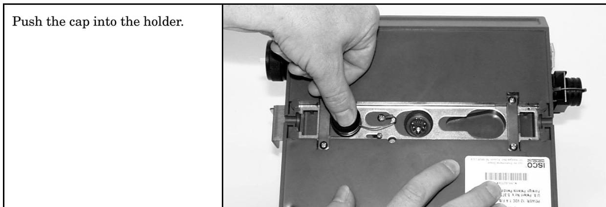
Figure 1-19 Flow Module - Pushing Cap into Holder
