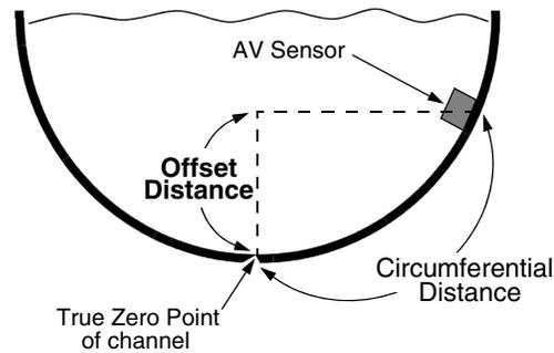
Figure 4-3 Zero Level Offset Measurement
