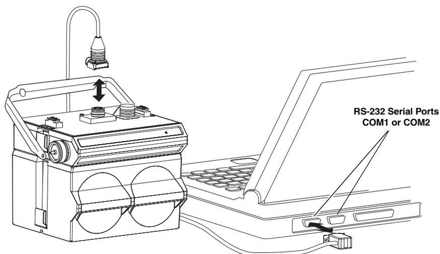
Figure 4-1 Flowlink connections
