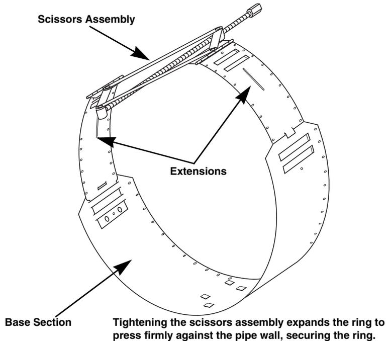
Figure 3-6 Scissors Ring adjustment
