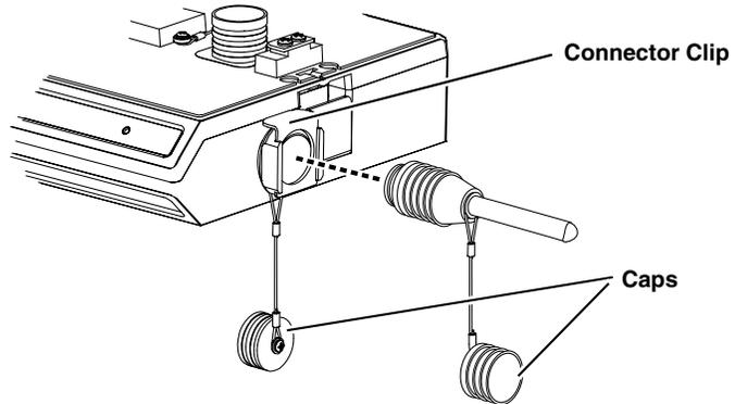
Figure 3-3 Connecting the AV Sensor
