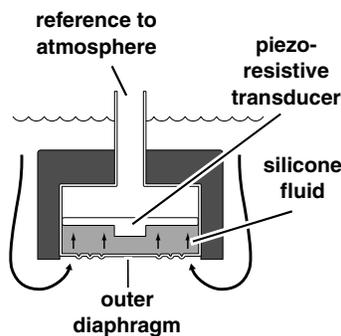
The AV Sensor's internal differential pressure transducer measures the liquid level. The transducer is a small piezo-resistive chip that detects the difference of the pressures felt on the inner and outer face.
