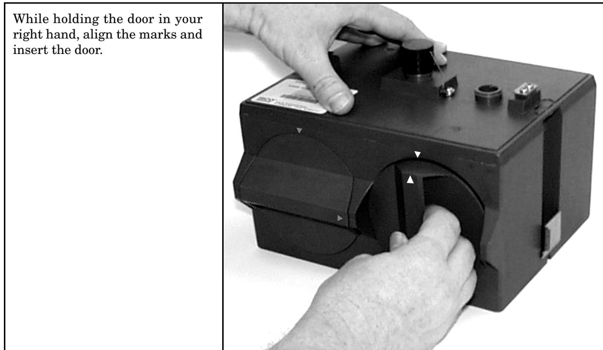
Figure 1-15 Battery Module - Aligning the Door
