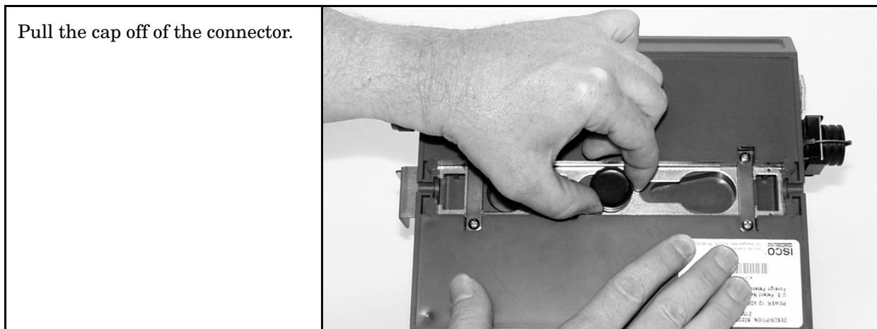
Figure 1-18 Flow Module - Uncapping the Connector
