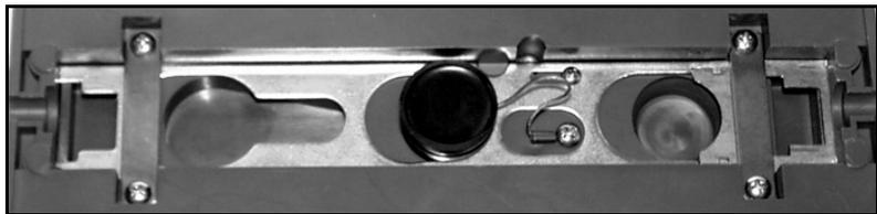
*Figure 1-7 Flow Module - Lower Connector, Capped*
