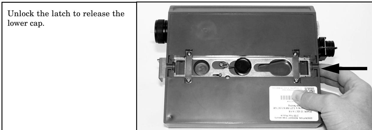
Figure 1-17 Flow Module - Unlocking the Latch
