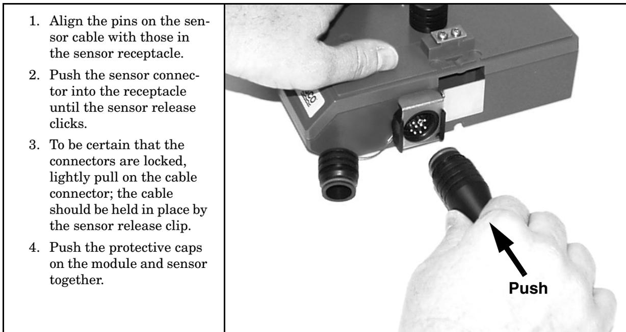
Figure 1-10 Flow Module - Connecting the Probe
