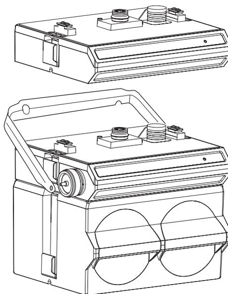
*Figure 3-2 Assembling a system (shown: 2 flow modules with 1 battery module)*
