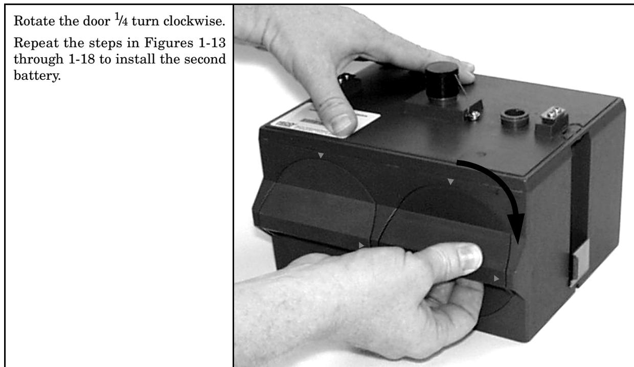
Figure 1-16 Battery Module - Closing the Door
