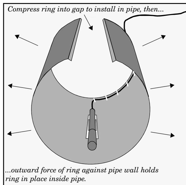
Figure 3-5 Sensor Installed on a Spring Ring
