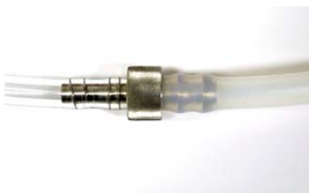
Figure 2-7 Attaching the suction line to the pump tubing
