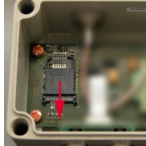
Figure 3. Open the SIM card holder
