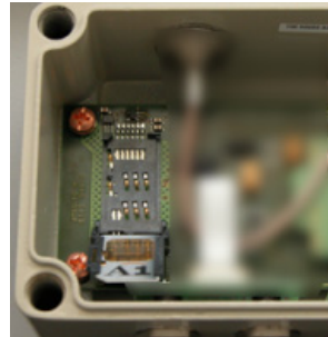
Figure 4. Insert the SIM card into the holder
