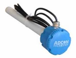
Depending on the length of the sensor up to 5 temperature sensors are available. The 30, 60, 90, 120 and 150cm probes have their first temperature sensor located at 15cm and every additional sensor with a spacing of 30cm, thus at 45, 75, 105 and 135cm resepctively.
