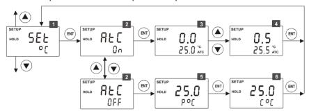
From measurement mode **press ENT key** to enter setup mode as described in section 5.1. The LCD shows the first screen of setup mode (**COF**). **Press ▲ or ▼ key** to select temperature settings screen (**SEt °C**).
