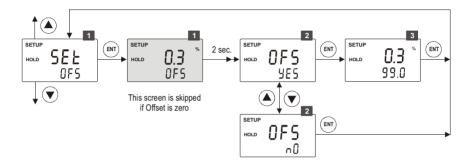
From measurement mode **press ENT key** to enter setup mode as described in section 5.1. The LCD shows the first screen of setup mode (**COFS**). **Press ▲ or ▼ key** to select offset settings screen (**OFS**).
