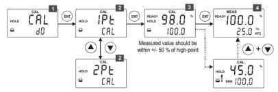
Calibration error occurs if measured value is not within +/- 50% of high-point during 1-point calibration
