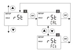
From measurement mode **press ENT key** to enter setup mode as described in section 5.1. The LCD shows the first screen of setup mode (**COF**). **Press** ▲ **or** ▼ **key** to select resetting screen (**rSt**).
