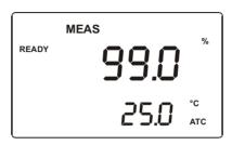
The mode indicator '**MEAS**' at the top of the display indicates that the Transmitter is in Measurement mode. The upper alpha-numerical display shows the measured dissolved oxygen value, while the lower display shows the temperature value. The indicator "%", "ppm" or "mg/l" at the upper right side of the display indicates the current measurement mode. (Refer section 5.2 for switching measurement modes)
