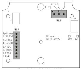
Figure 1: Outer Side of Back PCBA
