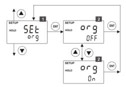
From measurement mode **press ENT key** to enter setup mode as described in section 5.1. The LCD shows the first screen of setup mode (**COF**). **Press ▲ or ▼ key** to select out of range settings screen (**SEt org**).
