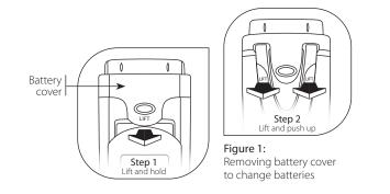
**Changing Batteries:** To remove batteries, lift up front battery cover and hold in position before lifting two sides of the pocket clip (Figure 1). Remove old batteries and replace with fresh ones. Note polarity as shown in battery compartment. No re-calibration is required after battery change since tester's non-volatile memory function retains calibration.
