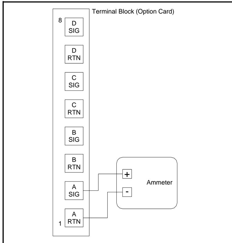
Figure 1-2: Ammeter Connection for Slots 1-6 (Output A)
