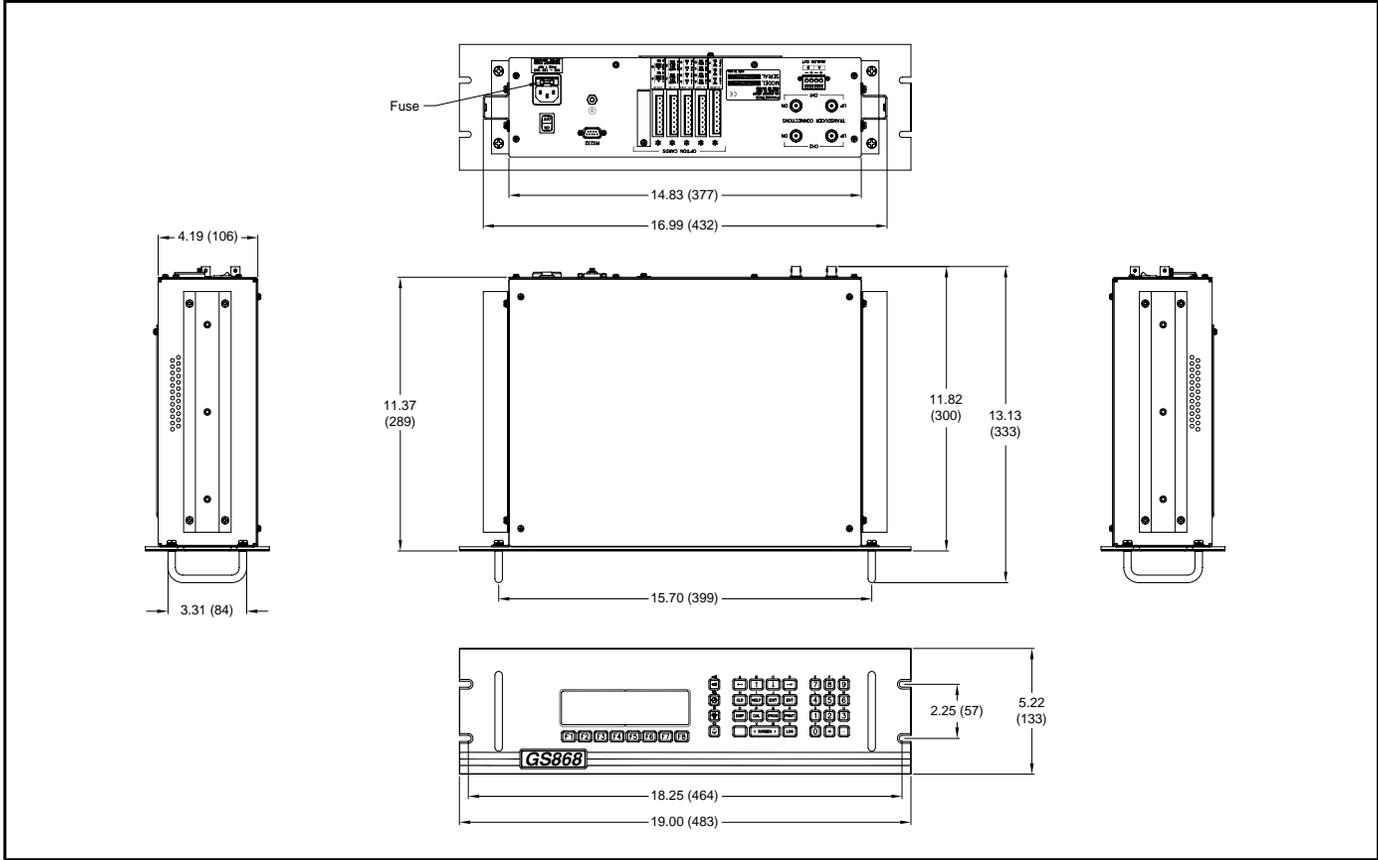
Figure B-1: Model GS868 Rack Mount Enclosure Dimensions - (ref. dwg #712-1078)
