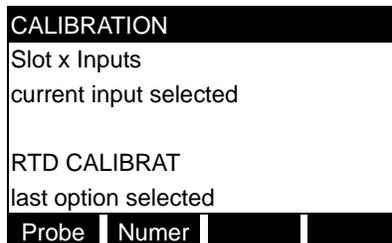
Press [F1] to select the Probe method of calibration, or [F2] to select the numeric method.
