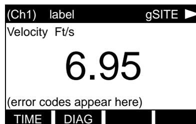
Press the [←] or [→] keys until DIAG appears on the option bar. Press the appropriate [F $x$ ] key to select this option.
