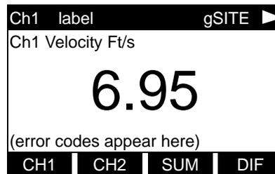
Press the [←] or [→] keys until the desired channel option appears on the option bar. Press the appropriate [F $x$ ] key to select this option.
