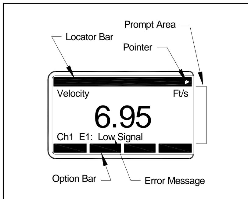
Figure 2-1: A Typical Display Screen
