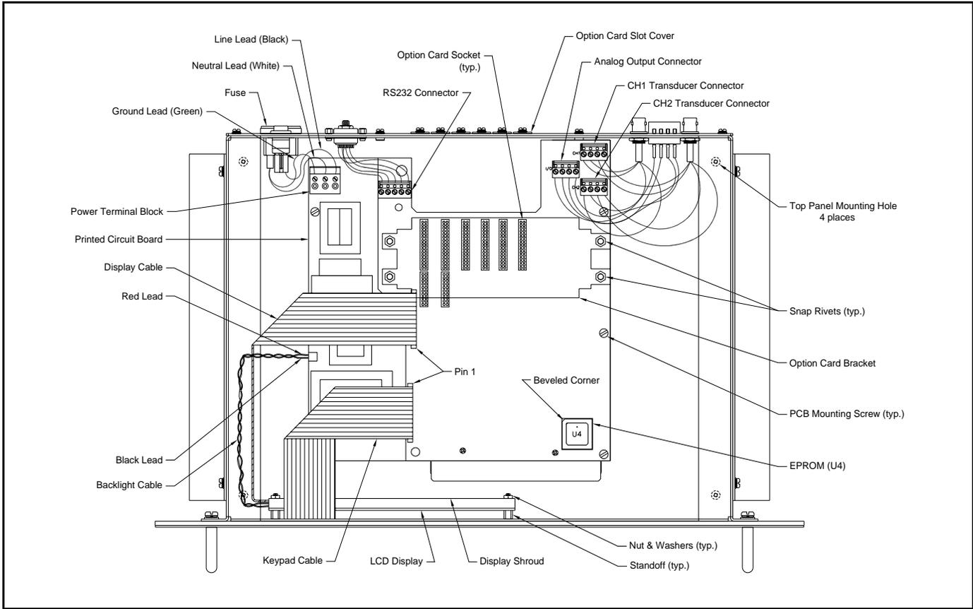
Figure B-2: Model GS868 Rack Mount Console Assembly - (ref. dwg #705-849)
