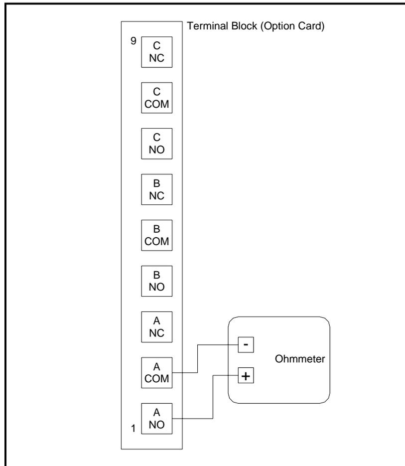
**Figure 1-4: Typical Ohmmeter Connections**
