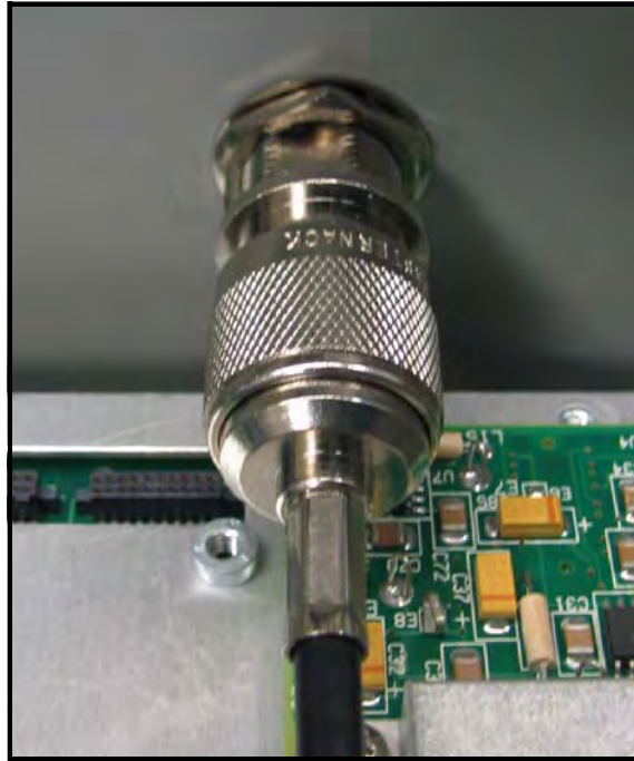
Figure 40: WI-FI Cable Antenna Connection
