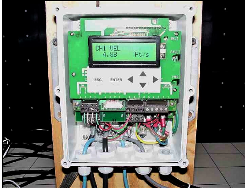
Figure 13: AT868 Properly Wired for CE Mark Compliance
