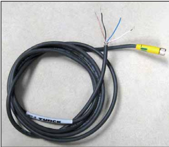
Figure 26: Four-Wire, IQ.probe Cable
