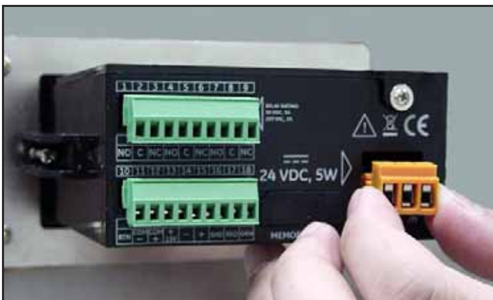
Figure 33: Removing the DC Power Connector
