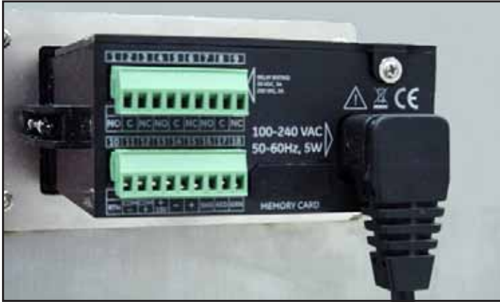
Figure 32: The AC Power Cable Installed
