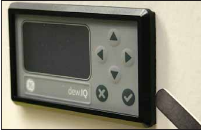
Figure 15: Checking the Gasket Compression
