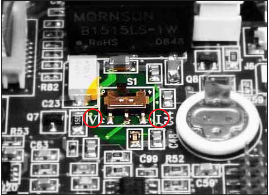
Figure 8: Switch S1 on the Main PC Board
