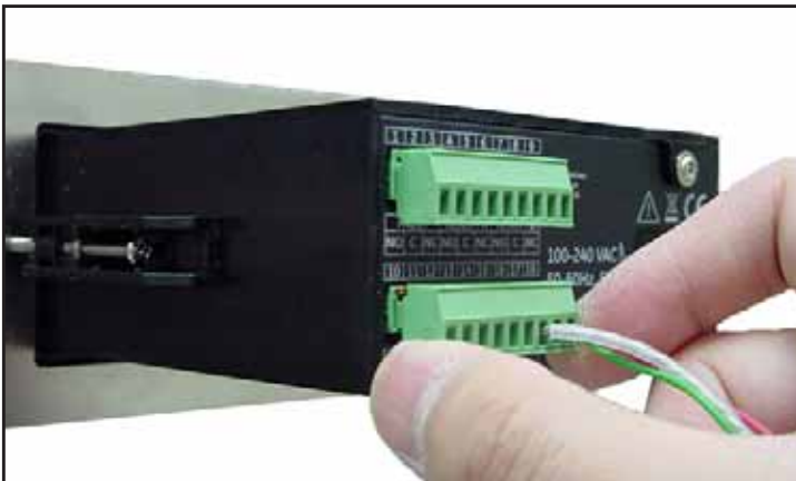
Figure 25: Reinserting the Connector into the Terminal Block
