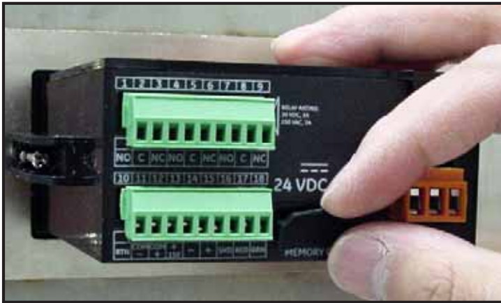
Figure 48: Pulling the Flexible Cover
