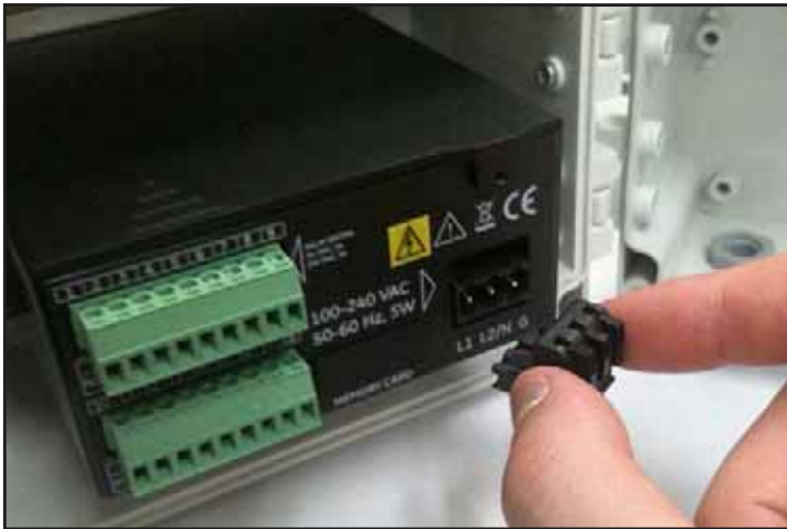
Figure 35: Removing the AC Power Connector
