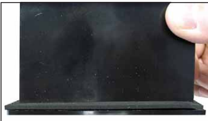
Figure 10: Installing the Gasket Behind the Display
