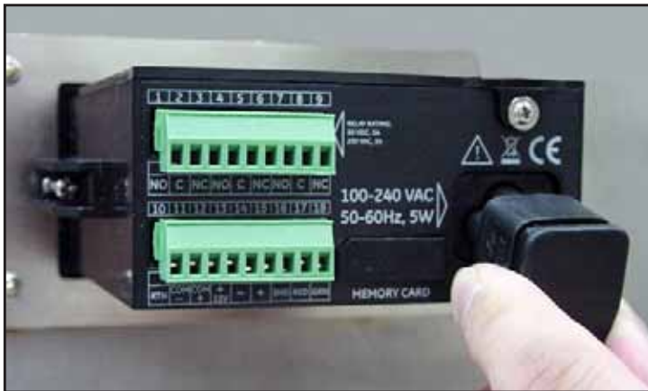
Figure 31: Inserting the AC Power Cable
