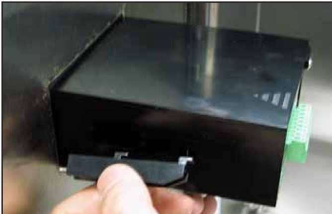
Figure 12: Installing the Mounting Brackets
