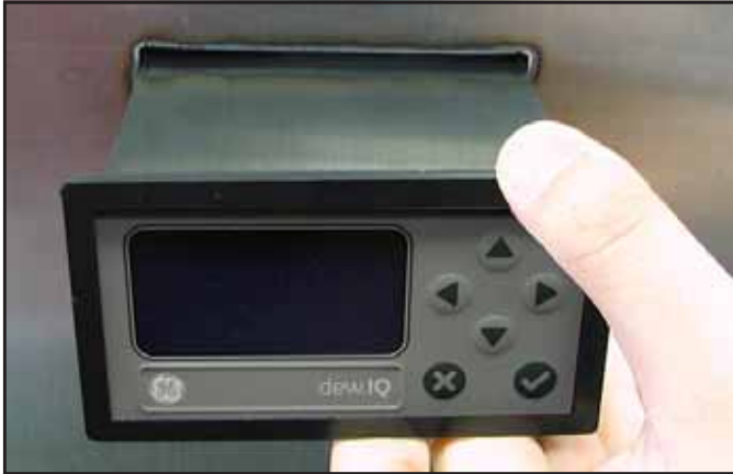
Figure 11: Sliding the dew.IQ into the Panel Cutout
