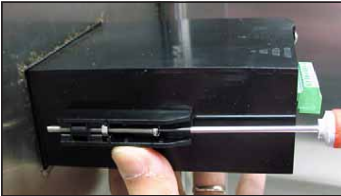
Figure 14: Securing the dew.IQ to the Panel
