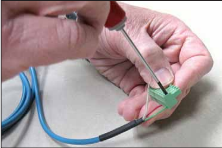
Figure 24: Making Probe Cable Connections to the Connector
