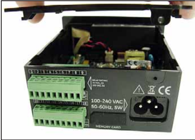
Figure 7: Removing the Cover
