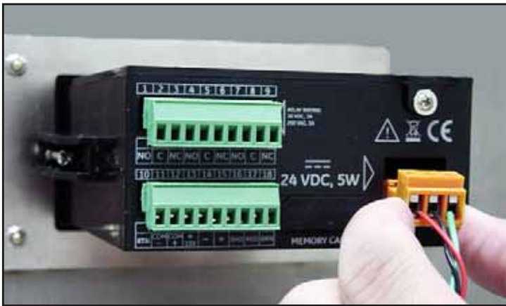
Figure 34: Reinserting the DC Power Connector
