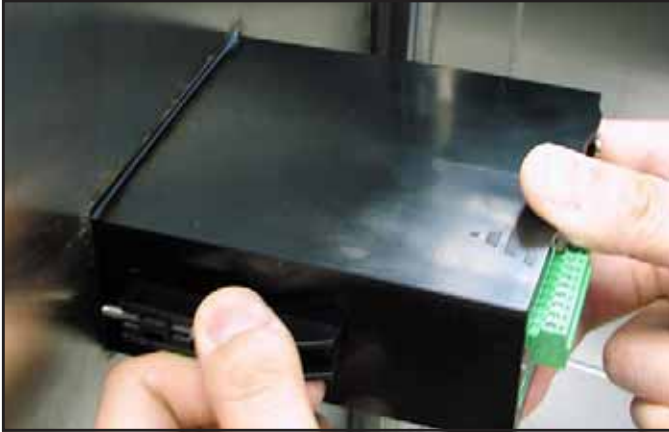
Figure 13: Locking the Mounting Brackets in Place
