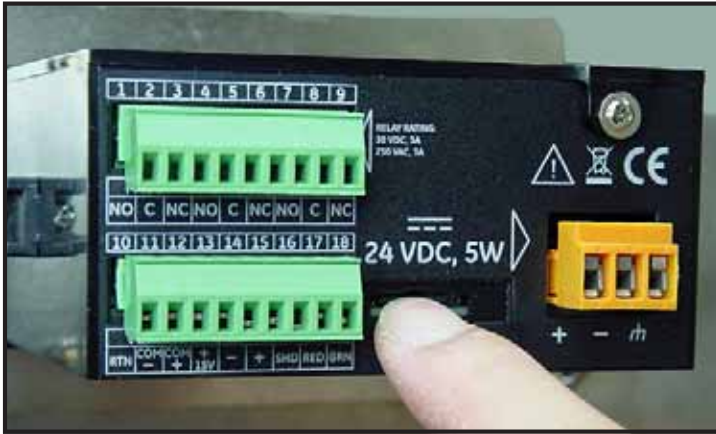
Figure 50: Pushing in on the MicroSD Card
