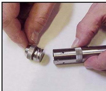
*Gently twist off the end cone, and then carefully remove debris.*
