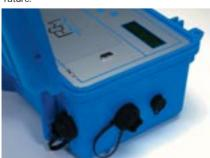
Using the Doppler ultrasonic measurement principle and the membrane-free pressure depth transducer, the sensor is not effected by fouling due to oil, grease and algal/bacterial growth. Doppler signals are assessed for their frequencies by a special software that calculates the true average velocity.
