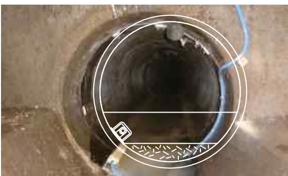
Hydrostatic measurement - flow level detection, e.g. in channels tending to sedimentation
