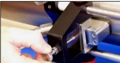
3. Set the second mounting block to the calculated spacing plus the initial scale number selected for the first mounting block.
