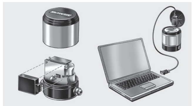
Add-on communication module (left), PC-IrDA connection (right)
