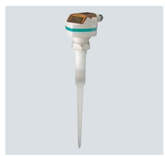
SITRANS Probe LR is a 2-wire, 6 GHz pulse radar level transmitter for continuous monitoring of liquids and slurries in storage vessels with nominal pressure and temperature, to a range of 20 m (66 ft).
