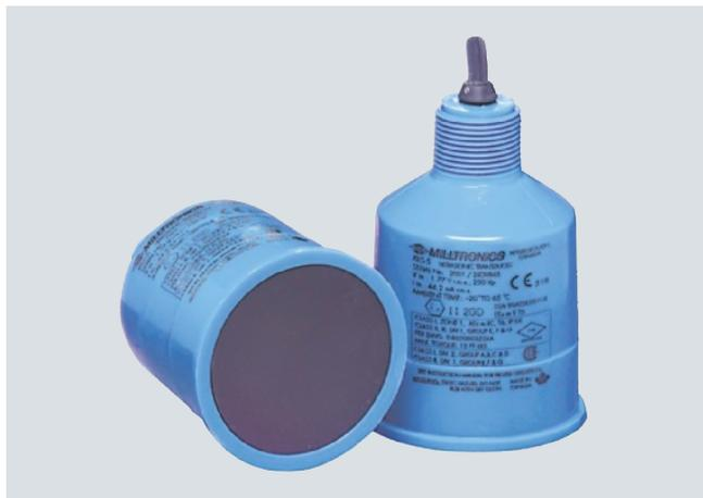
Echomax XRS-5 ultrasonic transducer provides reliable, continuous level monitoring of liquids and slurries in narrow lift stations/wet wells, flumes, weirs and filter beds using a beam angle of just 10° and a CSM rubber face.
