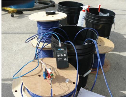
Figure 6-5 Presoaking the Vibrating Wire Transducers
