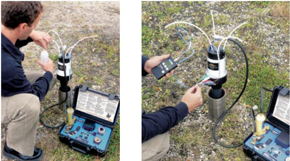
Figure 7-1 Testing Pumps and Transducers
