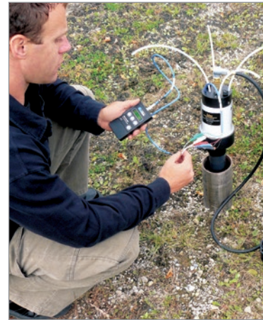
Collecting a sample from a dedicated DVP and taking pressure measurements with Model 404 Geokon Vibrating Wire Readout (above).
