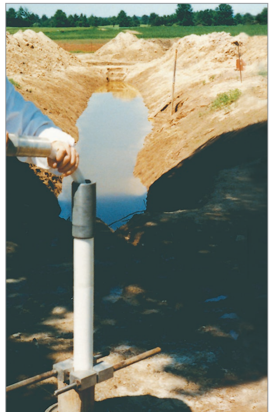
Underground oil pipeline leak assessment. Three 150 ft. (45 m) installations. Two point rising head permeability tests were conducted in each interval of the Multilevel System. (See diagram showing contaminant distribution at left.)
