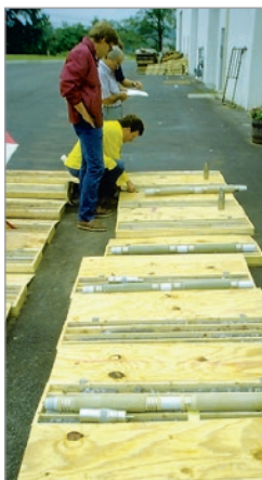
Using core logs to identify placement of Ports and Packers (left). Multi-Purge Manifold with transducers and dedicated pumps for four zone monitoring (right).
