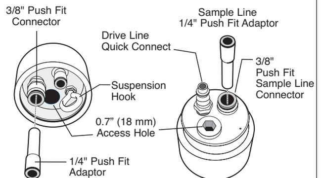
Wellheads come with two Push Fit Adaptors so that either 1/4" or 3/8" tubing can be used, as preferred.
