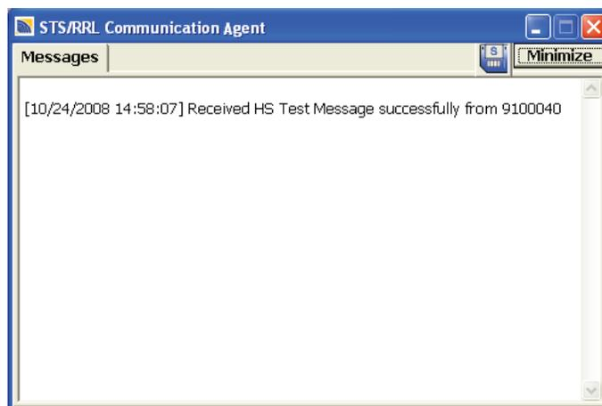
Figure 5-19 STS Communication Agent Showing a Successful Home Station Test
