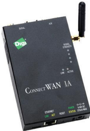
Figure 5-14 GSM Modem
