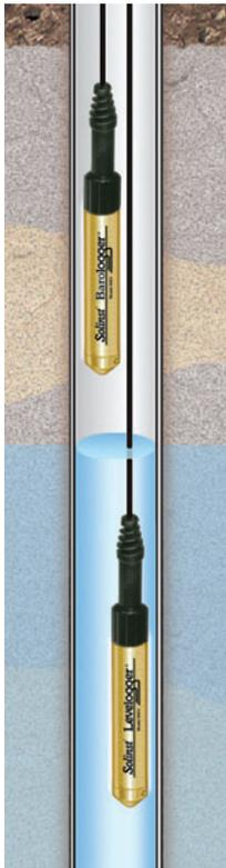
Figure 1-6 Levelogger and Barologger in Well
