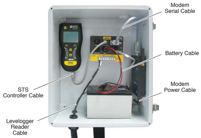
**Figure 6-3 Standard Remote Station Setup**
