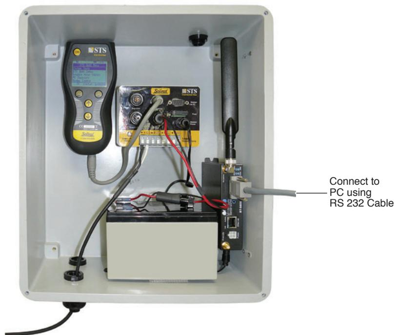
Figure 5-12 CDMA Modem Configuration Set-up
