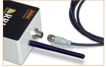
Power Cable Connection
