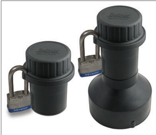
Well Caps can be permanently secured to the PVC casing using screws and the cap securely locked using a 3/8" (9.5 mm) shackle diameter lock
