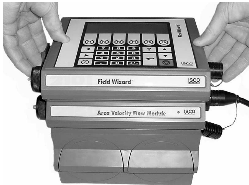
Figure 3-3 Field Wizard Connected to a 2150 Site
