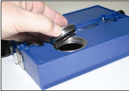
The SIM card is accessed via this waterproof twist-off cap located on the module's underside.
