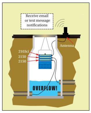
The 2103ci dial-out feature enables it to transmit a text message alarm to your digital cell phone or pager.
