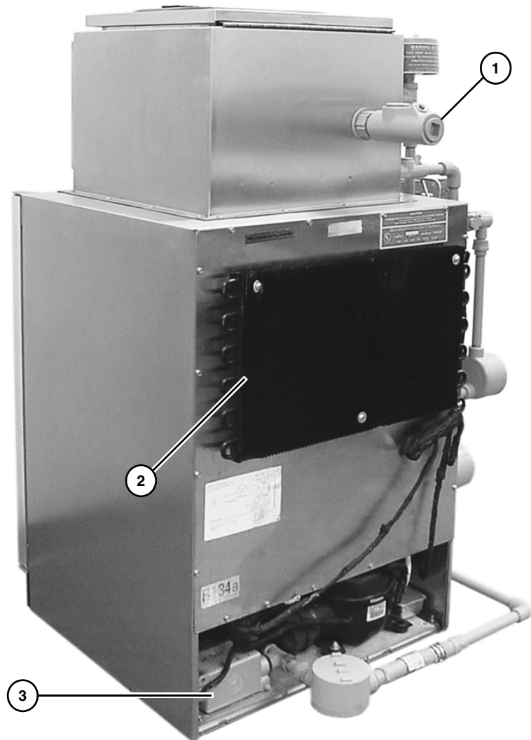
Figure 1-4 Rear view of 3700ZR showing condenser and conduit fitting
