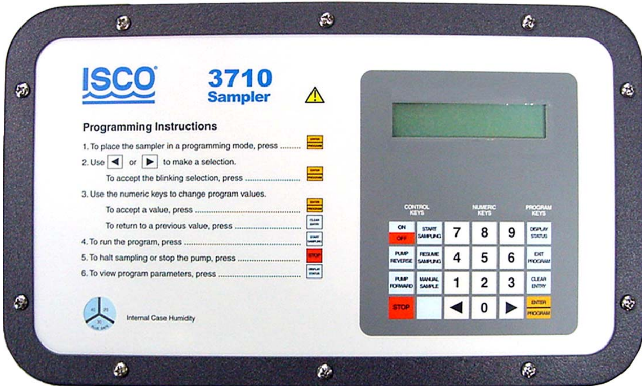
Figure 3-2 3710 Sampler Control Panel
