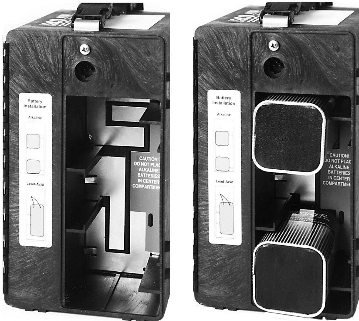
Figure 2-4 Installing Alkaline Batteries
