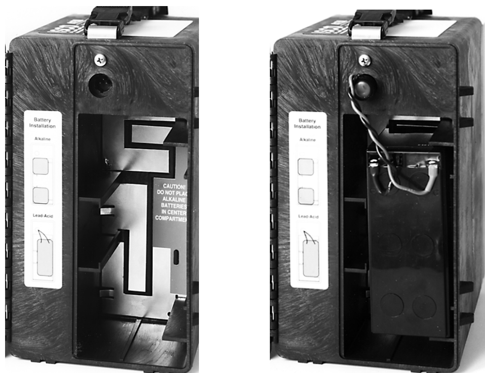
Figure 2-8 Installing the 947 Lead-Acid Battery
