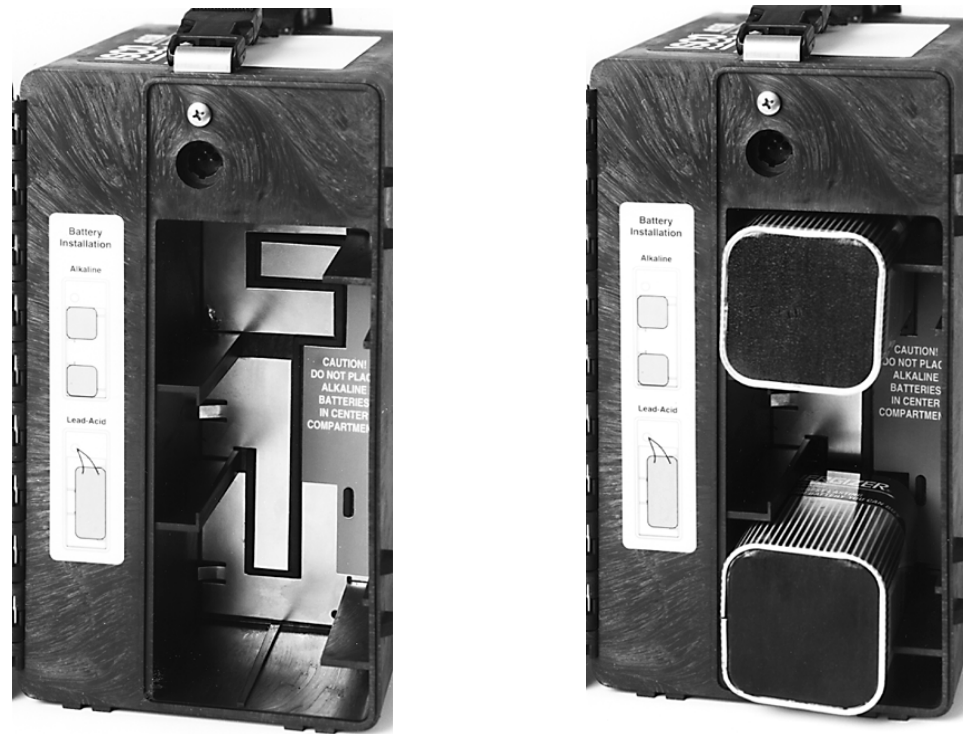
Figure 2-9 Installing Alkaline Batteries
