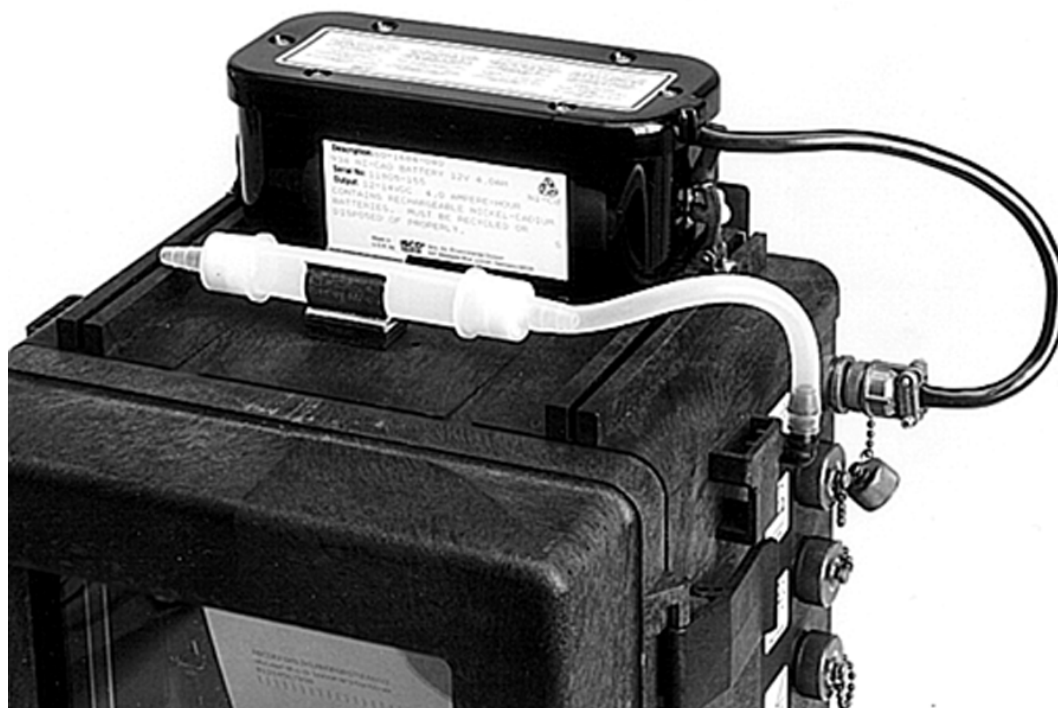
Figure 3-1 Nickel-Cadmium Battery Installed on a Flow Meter
