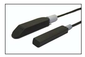
Isco offers both standard and low-profile area velocity sensors to meet your specific needs. The standard sensor (left) is most suitable in larger pipes and turbid flows with high concentrations of suspended solids and entrained air. An extended-range version of this sensor is available. See back.
