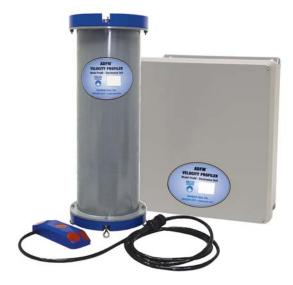
The ADFM electronics unit houses the signal processing, data logging, and data output electronics. The electronics unit is available as a NEMA 4X box enclosure, suitable for wall or console mounting in permanent applications, and a NEMA 6P cylindrical enclosure for use in manholes or other "wet" environments.
