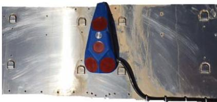
**Figure 23: Assembling the ring and mounting the sensor**
