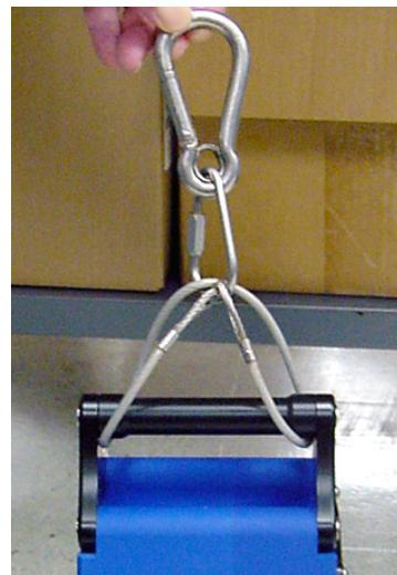
**Figure 4: accQpulse suspension harness**
