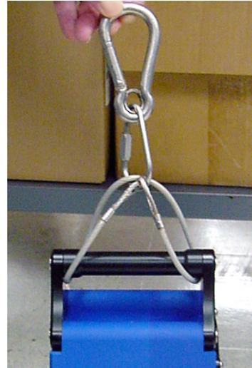
**Figure 4: accQpulse suspension harness**
