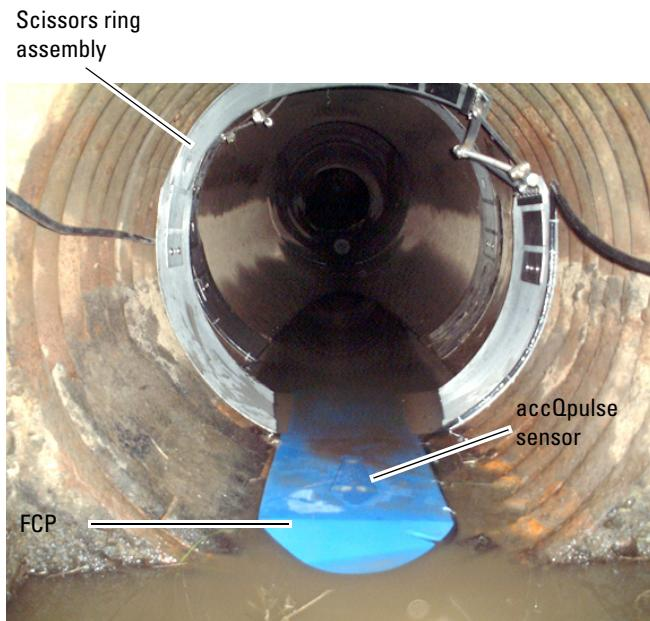
**Figure 14: FCP and Scissors ring installation**
