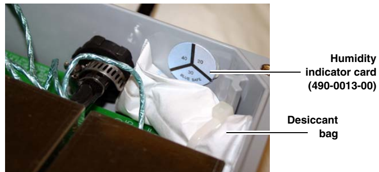
Figure 3-12 Location of desiccant bag and humidity indicator
