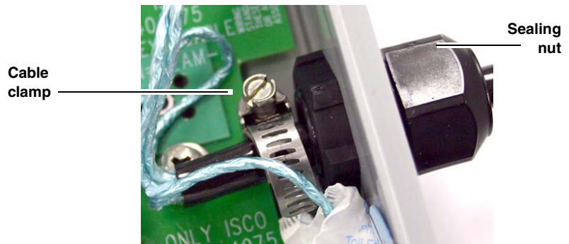
Figure 3-8 Release cable from clamp and cord-grip fitting
