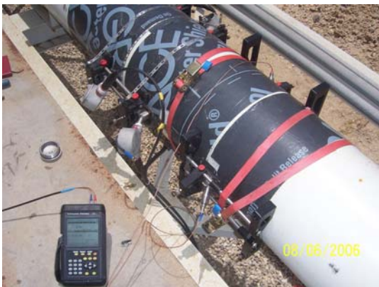
Fig. 1: Clamp-on gas flow meter PT878GC, available for hire or purchase.
