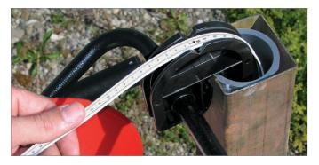
A Tape Guide allows depth measurements to be read at the marked position on the Tape Guide, to give reliable, repeatable, accurate depth measurements when profiling a well. The Tape Guide protects the tape from damage on rough edges of well casing.
