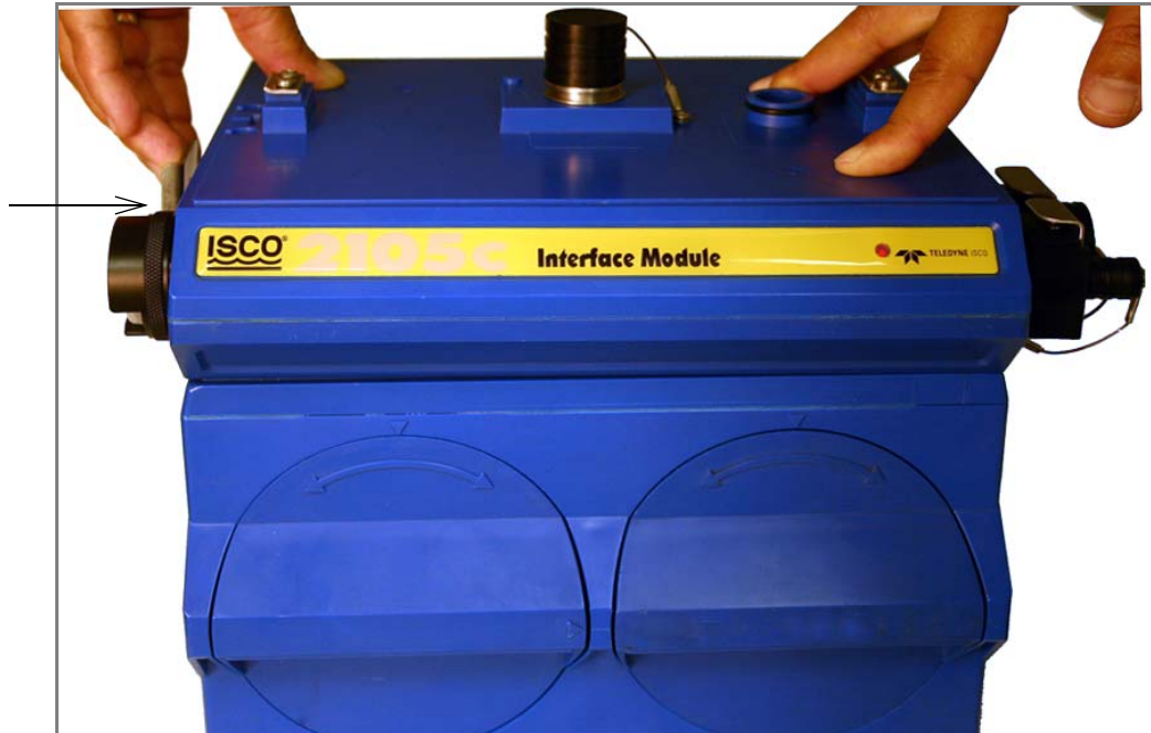
Figure 2-10 Aligning the modules
