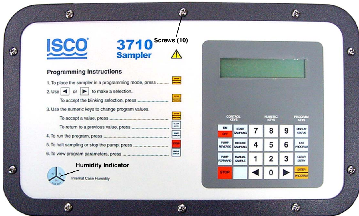
Figure 5-4 Location of 10 Screws on Control Box Bezel
