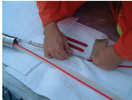
Figure 6-12 Using Sand Paper to Push Tubing onto Pump Stem
