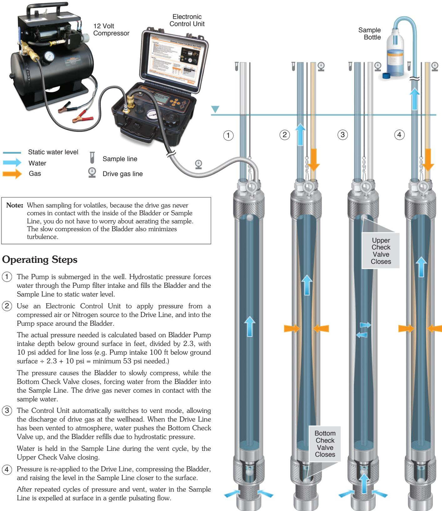
**Note:** When sampling for volatiles, because the drive gas never comes in contact with the inside of the Bladder or Sample Line, you do not have to worry about aerating the sample. The slow compression of the Bladder also minimizes turbulence.
