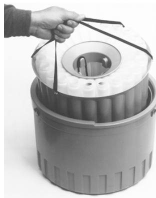
Removing Bottles From the Compact Sampler
