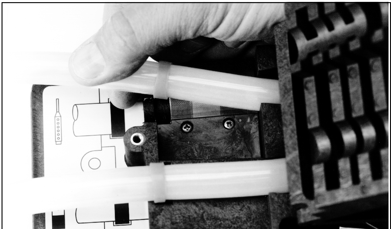
Figure 8-2 Placing the Pump Tube in the Liquid Detector
