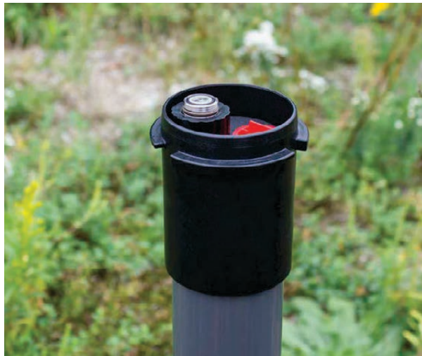
Remove Existing Levellogger Installation
