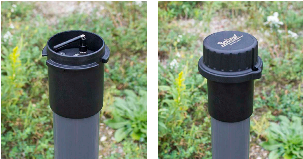
Figure 6-9 Install the Well Cap
