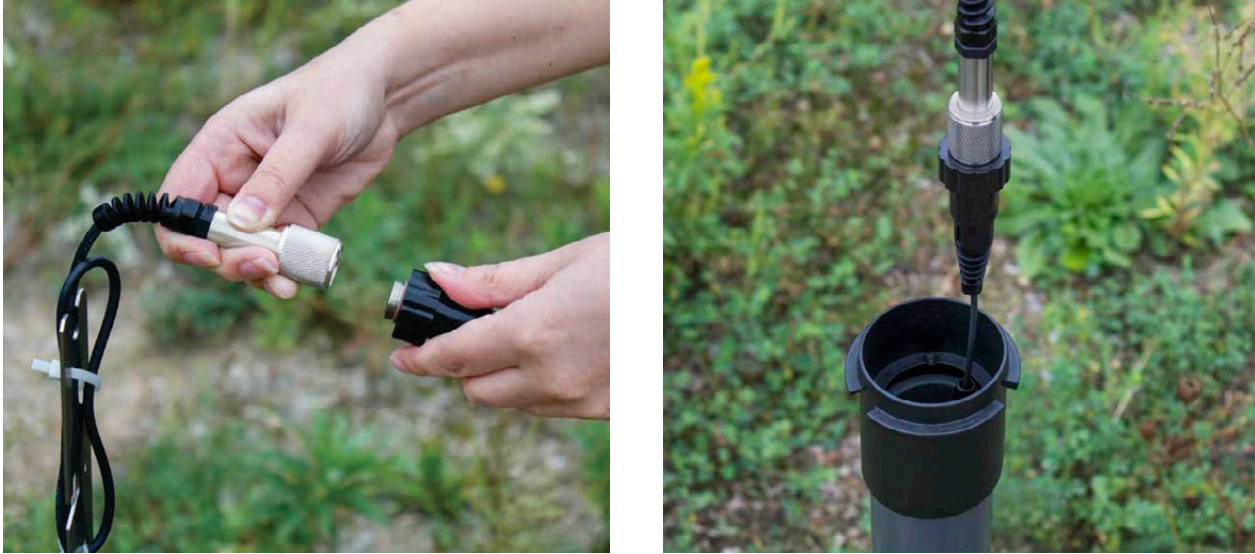
Figure 6-5 Connect the Direct Read Cable and Levellogger
