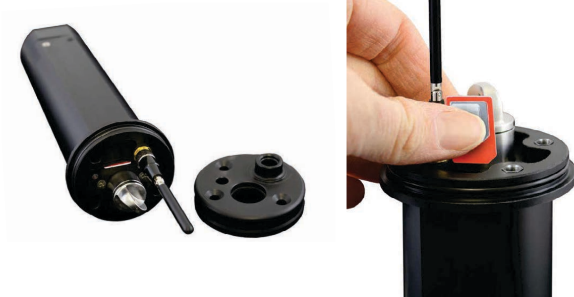
Figure 2-3 Installing the SIM Card
