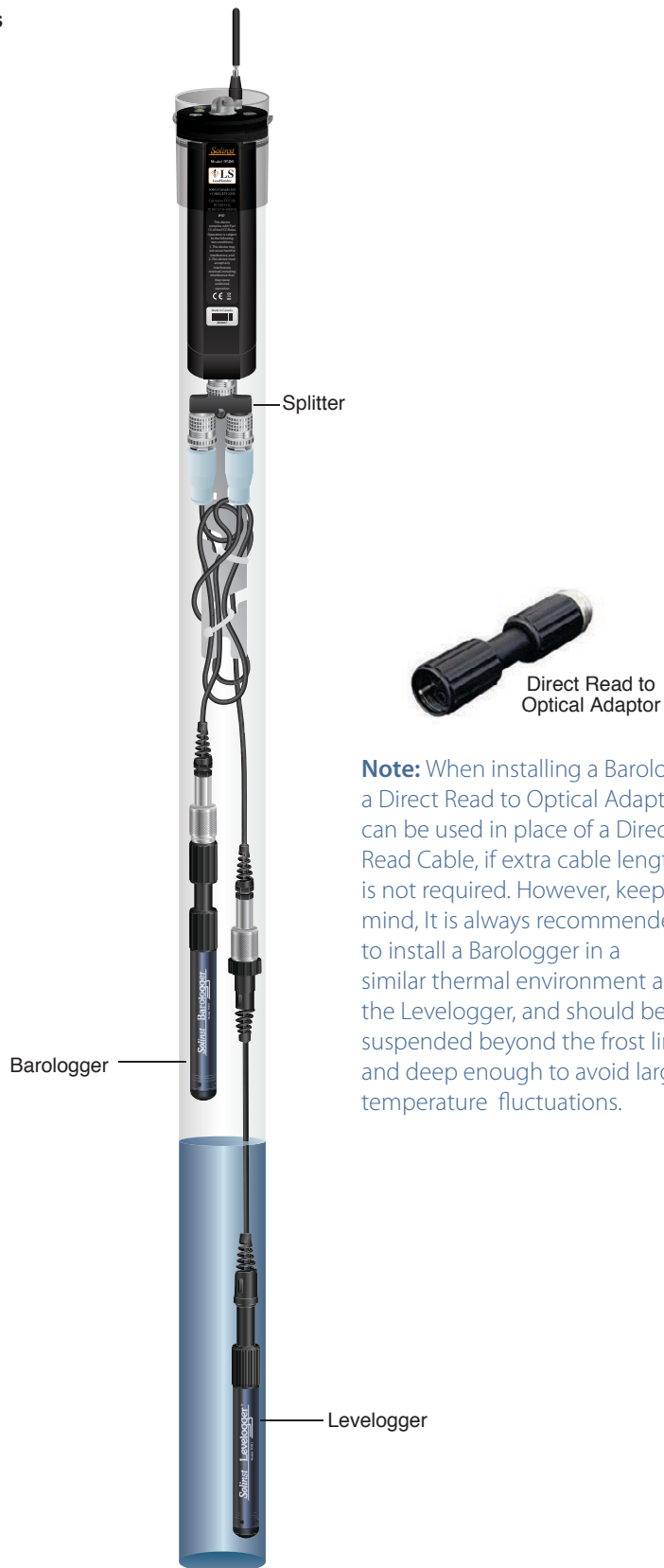
Figure 6-11 Levellogger and Barologger Installation (Reader Cable Connections Staggered)
