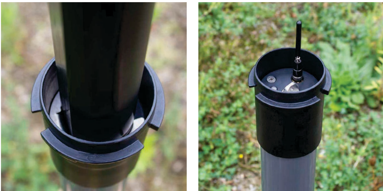
Figure 6-8 Lower the LevelSender into Position
