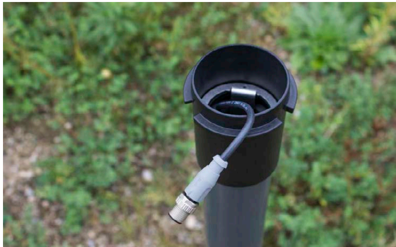
Figure 6-6 Lower the Assembly into the Well
