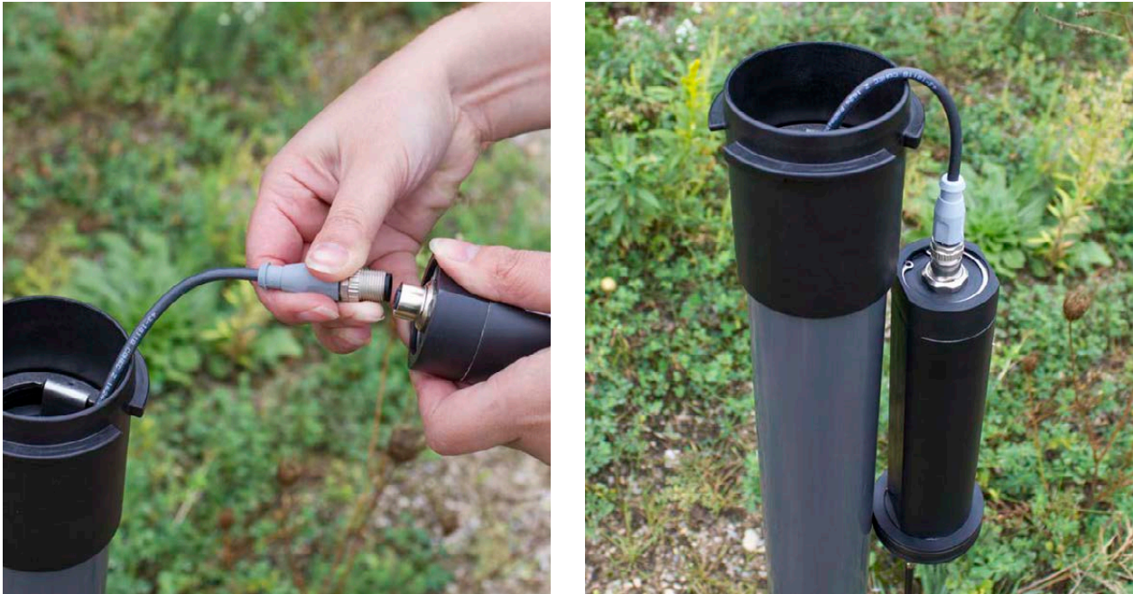
Figure 6-7 Connect the Reader Cable to the LevelSender
