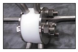
Run the cotter pin through the hole in the center bolt and bend the long leg around one of the ridges on the castle nut.
