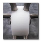
Run the bolt with pinhole downward through the buoy frame. Place a lock washer and the castle nut onto the bolt. Use a pair of 1-1/8" or adjustable wrenches to tighten the castle nut.
