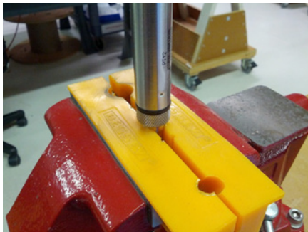
Cabled Sensor—gripping on swage
