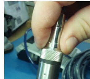
Properly completed—black ring uncompressed
