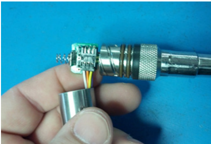
Connector connected properly
