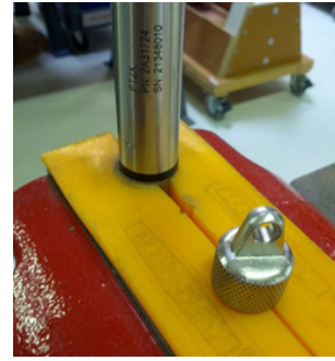
Cableless Sensor—gripping on knurled area
