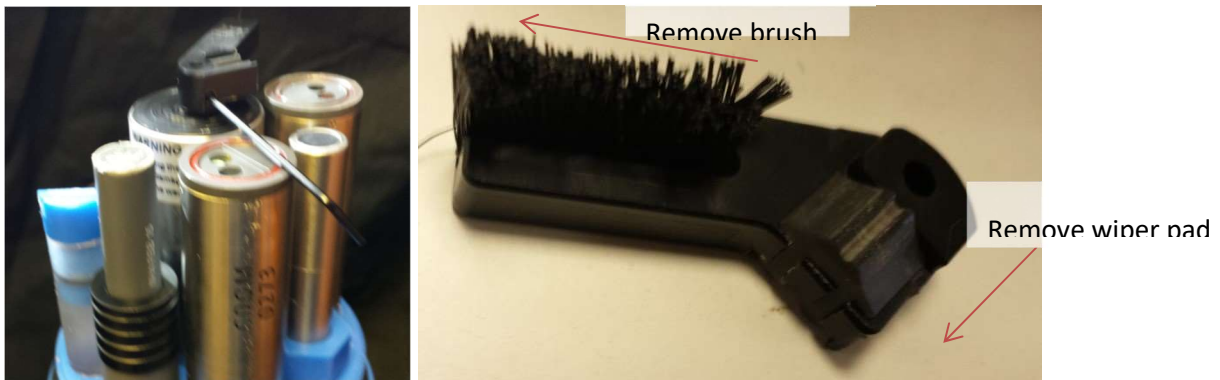
Figure 21. (a) Location of set screw for removing the wiper (b) brush arm with wiper pad and brush highlighted
