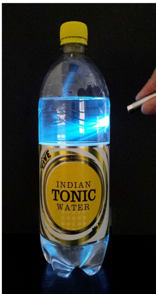
Figure 1: Example of quinine sulphate molecules in tonic water emitting blue light when exposed to high energy (UV) light.
